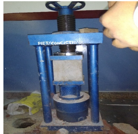
Fig. 2: Compressive strength test with machine setup
