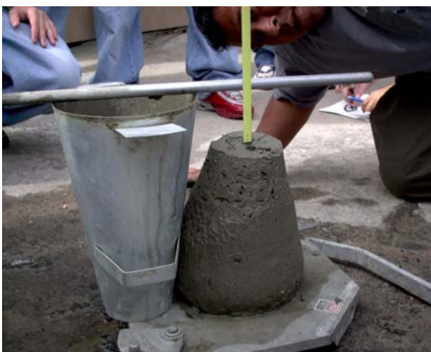
Fig. 1: Slump test apparatus along with slum measurement
