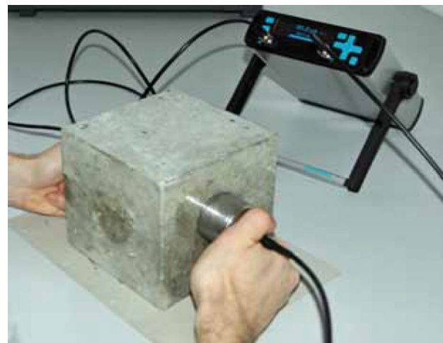
Fig. 3: Pulse velocity test on concrete cube
